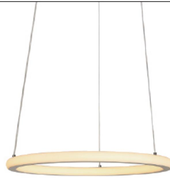
030M3-468 Double sides Ring light is built by Alu. extrusion fixture with Silicone lens. It's creating smooth and comfort lighting. The light sourced are Osram LED in 80+ or 90+ Ra available. Color temperature options from 2700K to 6500K, Dual white, Dim2Warm at WW+NW aviable. Variouse dimmable functional.
